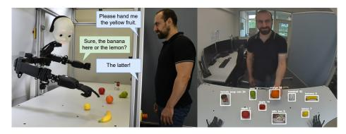
**Fig. 1.** The robot uses a grounded LLM to understand and correctly react to ambiguous conversation by the user. This can include, for example, actions such as looking and pointing at objects in order to clarify its or the user's intentions.
