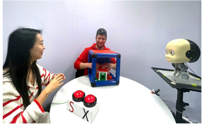
Fig. 1. Experimental setup. Two participants adopt the roles of a guide (left) and an actor (center) while the iCub robot (right) observes their gameplay. The actor inserts an object into the sorter following the guide's instructions.
