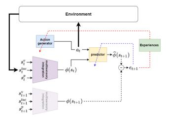
**Fig. 5** Proposed model for developing the active self in artificial agents.  $s_t^{\gamma}$ ,  $s_t^{rac}$ ,  $s_t^{\rho}$  denote raw visual, tactile, and proprioception input at time t respectively. The blue and red arrows denote the source of data affecting the learning of the target module: blue for the *predictor* and red for the *Action generator*.
