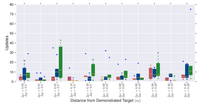
Fig. 8. Comparison between different approaches in grasping the cylinder. The result shows a small deviation from the original position of the object during demonstration results in a DMP failure. PI^2 shows the best performance, while eNAC requires the highest number of updates.
