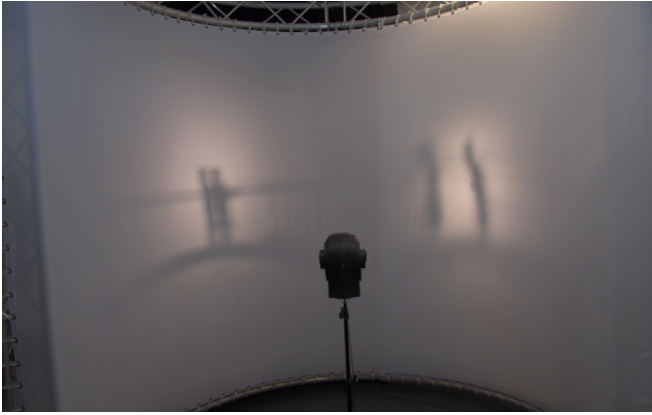
Fig. 5: Lab setup of the Soundman head in front of loudspeakers behind a screen. The positions of the speakers are highlighted with external light. See also [33].
