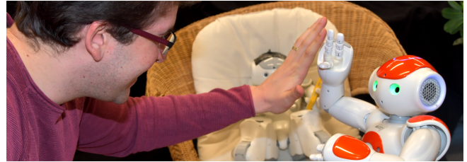
Fig. 1. An HRI illustration where a NAO robot will continually learn facial expressions through close interactions using the proposed approach.
