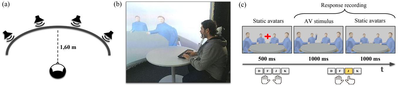
Fig. 1. Behavioural study on audio-visual localization: (a) Immersive experimental setup with acoustically transparent concave projection screen (b) Subject selecting a position via a keyboard (c) Schematic illustration of one trial of the AV localization task.
