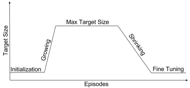
Fig. 4. Exemplary target size adaptation: during the 20 first steps, the size is not changed as the current reaching ability of the learner is evaluated. Usually the target is not reliably reached which results in the target growing to its upper size limit. Once the target is reliably reached, it begins to shrink gradually. Finally, when the agent reliably reaches the target, fine tuning on the non-simplified target prevents learning artifacts from simplified instances.
