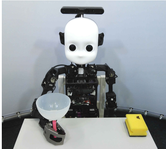
Figure 7.12: Cleaning scenario with the NICO robot. Our scheme is composed of 2 objects, 3 locations, and 7 action classes (Cruz et al., 2016b).
