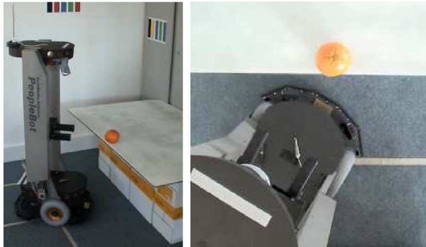
Fig. 1. The PeopleBot robot during the docking manoeuvre. On the left are visible the camera pointing downward (mounted underneath the top plate) and the black grippers. Right, the scenario from above. The black grippers are hardly to be seen over the dark robot's base; a fraction of the camera can be seen bright.
