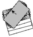
Figure 5: The ten steps of the learnt ‘go’ behaviour, as the robot starts to turn away from the wall.
