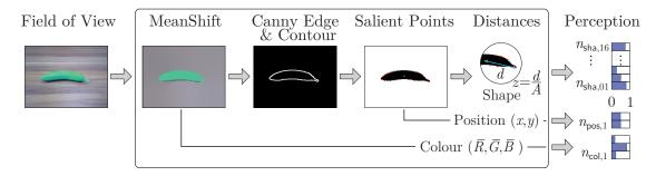
Figure 3.6: Schematic process of visual perception and encoding. The input is a single frame taken by the NAO camera, while the output is the neural activity over N neurons, with N being the sum over shape + colour + position features.
