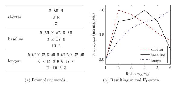
Figure 5.8: Comparison of mixed  $F_1$ -score for different timescale values over shortened and prolonged average word lengths. The timescale ratio are varied for  $\tau_{Cf}/\tau_{IO}$  layer only. For the first setup, all words have been artificially halved in length (to a minimal length of one phoneme) and for the second setup, all words have been doubled in length. Results have been normalised for each setup to increase readability.
