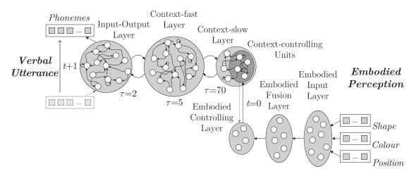
**Figure 5.1:** Architecture of the EMBMTRNN model: a *Multiple Timescale Recurrent Neural Network* (MTRNN) extended by embodied perception from the scene. A sequence of phonemes (verbal utterance) is processed over time, while the perceived embodied and situated information is constantly present.
