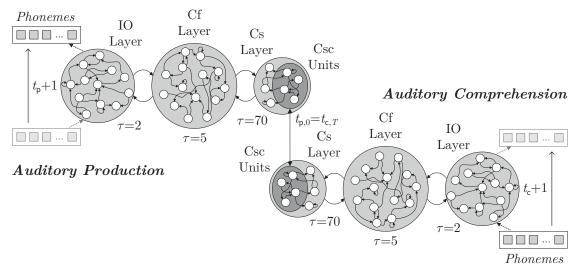
**Figure 6.8:** Architecture of the CPUNIMTRNN model: a *Multiple Timescale Recurrent Neural Network* (MTRNN) with context bias connected via associative links with an MTRNN with context abstraction. In a closed loop a sequence of phonemes (verbal utterance) is produced over time and comprehended over time.
