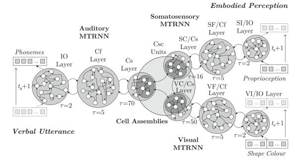
Figure 6.11: Architecture of the multi-modal MTRNN model, consisting of an MTRNN with context bias for auditory, two MTRNNs with context abstraction for somatosensory as well as visual information processing, and *Cell Assemblies* (CAs) for representing and processing the concepts. A sequence of phonemes (utterance) is produced over time, based on sequences of embodied multi-modal perception.
