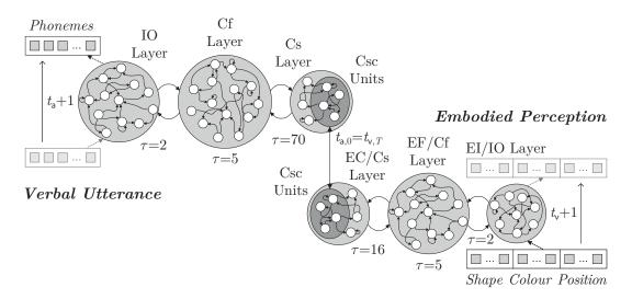
**Figure 6.4:** Architecture of the SO-UNIMTRNN model: a *Multiple Timescale Recurrent Neural Network* (MTRNN) extended by embodied perception from the scene. A sequence of phonemes (verbal utterance) is processed over time after the *self-organised* semantic context of a sequence of perceived embodied and situated information has been associated.
