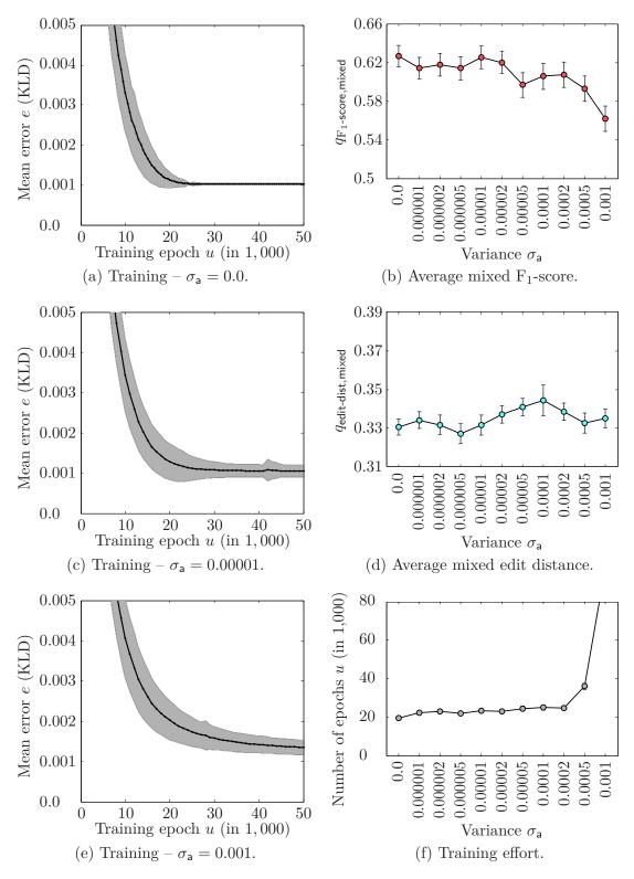
Figure 5.12: Influence of perturbing output sequences by normalised Gaußian jitter on training and generalisation: mean error (KLD) with confidence interval (standard error) over training epochs u (a, c, e), comparison of varied variance parameter  $\sigma_a$  (b, d, f), with error bars reflecting the standard error, each over 100 runs.
