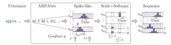
Figure 5.3: Schematic process of utterance encoding. The input is a symbolic sentence, while the output is the neural activity over  $|I_{\rm IO}|$  neurons times  $T_{\rm a}$  time steps.
