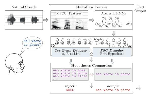
Figure 3.2: General architecture of a multi-pass decoder.
