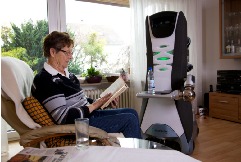
Figure 2.4: A robot monitoring and assisting an elderly in a home environment. In this example, the Care-O-Bot 3 robot (Reiser et al., 2013) offers water to the elderly after detecting that she has not drunk enough water for a long time.
