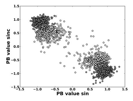
Figure 5.8: Scatter plot of PB values for the two test sequences. The PB values obtained for the first sequence (sin) are plotted against the PB value for the second sequence (sinc). Gray dots represent values obtained with the classical and white dots values obtained with the adaptive algorithm.
