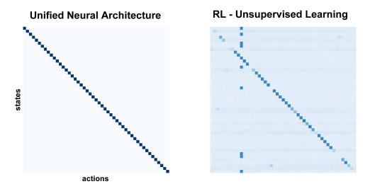
Figure 4.13: Comparison of rearranged Q tables. Every invariance (state) is linked to a single adequate action after learning with the unified architecture (left). However, this is not the case for RL following unsupervised learning (right). Some state-action pairs are not correctly learned. Strong weights are displayed dark.
