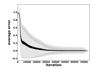
Figure 4.5: Average (1000 runs) error for a  $3 \times 3$  world. The network is trained with the novel unified architecture (Ch. 4.3.1). The mean squared error decreases monotonically. Only the errors of movements that actually reach the target are considered. Invalid actions, as well as unsuccessful ones, are left out. The gray shaded area delineates  $\pm 1$  STD.
