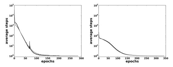
Figure 5.10: Semi-log plot showing average steps per epoch comparing classical (left) to adaptive (right) RNNPB. The average number of steps per epoch of the sin sequence are shown in black and for the sinc sequence in gray.
