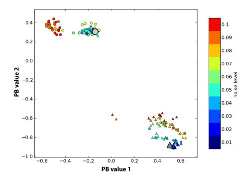
**Figure 5.15: Uni-modal noise tolerance.** Uniformly distributed noise of increasing levels (color coded) is only added to the visual prototype time series for the light-weight circle and the heavy triangle. The PB values are determined and marked with a matching symbol. The light gray circle and dark gray triangle show the PB values obtained during training without noise.
