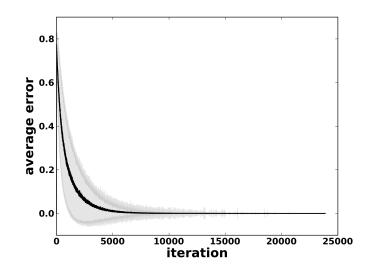
Figure 4.8: Average (1000 runs) error for a  $4 \times 4$  world. The network is trained using cubic RL (Ch. 4.3.2). The mean squared error decreases monotonically. Only the errors of movements that actually reach the target are considered. Invalid actions, as well as unsuccessful ones, are left out. The gray shaded area delineates  $\pm 1$  STD.
