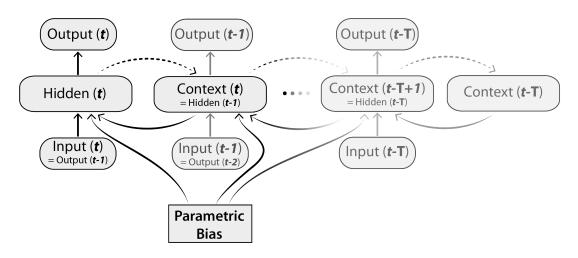
Figure 5.1: Network architecture. The Elman-type Recurrent Neural Network with Parametric Bias (RNNPB) unfolded in time. Dashed arrows indicate a verbatim copy of the activations (weight connections set equal to 1.0). All other adjacent layers are fully connected. t is the current time step, T denotes the length of the time series.
