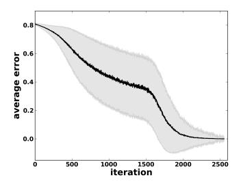
Figure 4.10: Average (1000 runs) error for a  $4 \times 4$  world. The network is trained using unsupervised learning followed by RL (Ch. 4.3.3). Only the MSE during RL is shown. The error decreases in two phases. This is probably due to the insufficient acquisition of the state space during unsupervised learning. Only the errors of movements that actually reach the target are considered. Invalid actions, as well as unsuccessful ones, are left out. The gray shaded area delineates  $\pm 1$  STD.
