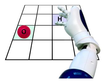
Figure 4.1: Reaching Scenario. The 2-D world is discretized. Hand (H) and object (O) are located at specific positions within this grid. The task for the simulated agent is to reach for the object with a single movement. If hand and object are both shifted by an identical displacement vector, their relative position with respect to each other does not change. Hence, another goal of the agent is to identify those invariant positions.
