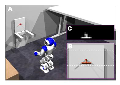
Figure 3.2: Nao robot in front of the docking position. (A) Webots simulation environment representing a domestic situation. (B) Camera view from the robot. The landmark (red) is located within a white dotted rectangle reflecting the region that serves as an input to the network. (C) Input image I after preprocessing.
