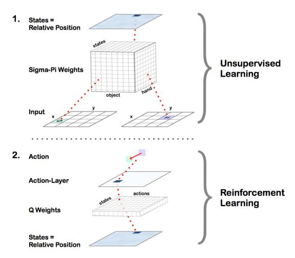
Figure 4.4: Two separate neural architectures. First, unsupervised learning is used to self-organize the state space of possible hand-object relations. Once this learning has been completed, a second RL algorithm links the acquired knowledge of the first procedure to suitable actions. Please see text for details. Only one example connection between any two layers is shown.
