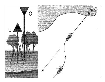
Figure 3.1: Leading lights for nautical navigation. The lower (U) leading light in conjunction with the upper (O) one can be exploited for navigation. Depending on the observed relation the tillerman can deduce how to navigate to reach the destination. Once the tips of the triangles point at each other he has to maintain the current bearing. For further details please see the text. Picture taken from Schult (2008).
