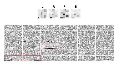
Figure 3.5: Receptive fields of hidden feature neurons (bottom) and action neurons (top) after 2000 steps of training. The RFs of the action units correspond to left (L), right (R), forward (F) and backward (B) movement. The RFs of the feature neurons that have the strongest contribution on the action units for L,R & F are framed in red. Strong weights are displayed dark.
