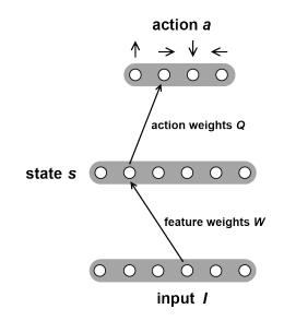
Figure 3.3: Schematic overview of the network architecture. Only one example connection between any two layers is shown.
