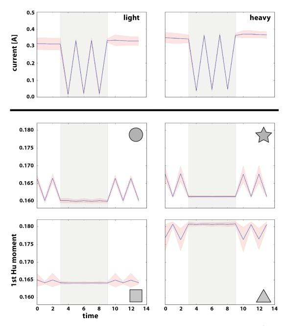
Figure 5.7: Training data. The mean values of the two weight conditions (light and heavy, top) and the four visual conditions (matching symbols, bottom) are shown. These mean time series are used as prototypes for training the RNNPB. Gray shaded areas represent the up and down movement, whereas back and forth movements are unshaded. The red area surrounding the signals delineates two standard deviations from the mean.
