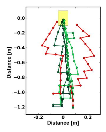
Figure 3.6: Sample trajectories of the robot. Different shades of green represent successful trials and red failures. The yellow docking region measures  $8 \times 20$  cm.
