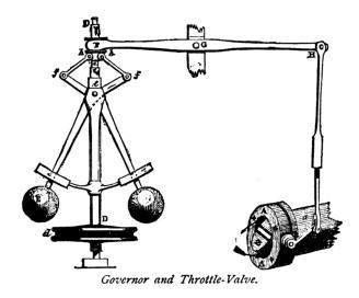
Figure 2.3: Watt's centrifugal governor. Example utilized by van Gelder to strengthen his dynamical hypothesis<sup>32</sup>.
