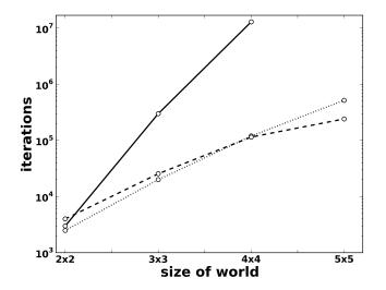
Figure 4.14: Semi-log plot depicting training iterations of the different architectures depending on the size of the world. Comparing the three models reveals that the increase of iterations is much more rapid for the unified architecture. The solid line shows the iterations of the unified architecture, the dashed line unsupervised learning followed by RL and the dotted line cubic RL.
