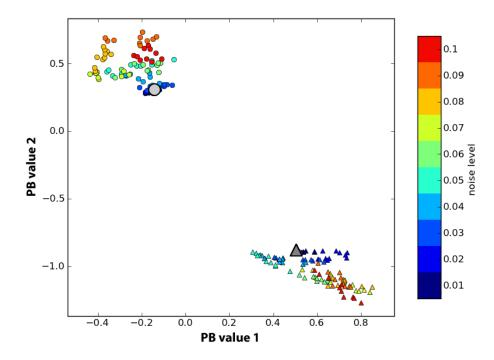
Figure 5.16: Bi-modal noise tolerance. Uniformly distributed noise of increasing levels (color coded) is added to both (visual and proprioceptive) prototype time series for the light-weight circle and the heavy triangle. The PB values are determined and marked with a matching symbol. The light gray circle and dark gray triangle show the PB values obtained during training without noise.
