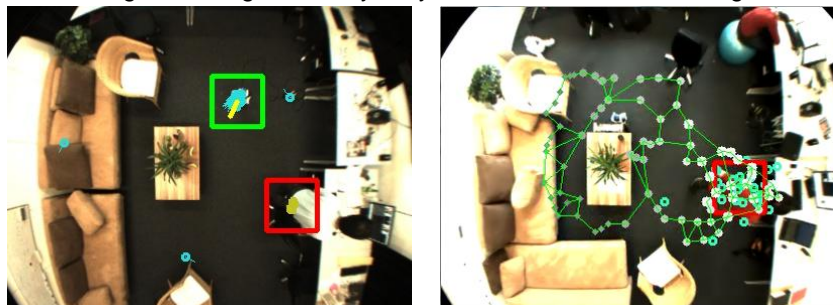
Figure 1. Ceiling-camera view of an apartment Left: A person (at red box) and a robot (at green box) are localized. The green spots are particles for the robot and the yellow for the user. Right: The units and the links of the built cognitive map.
