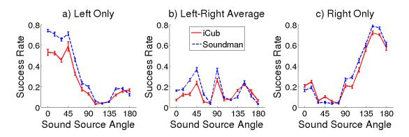
Figure 5.6: Average success rates of the DASR system. Results obtained with both robotic heads for the frontal  $180^{\circ}$  on the azimuth plane.
