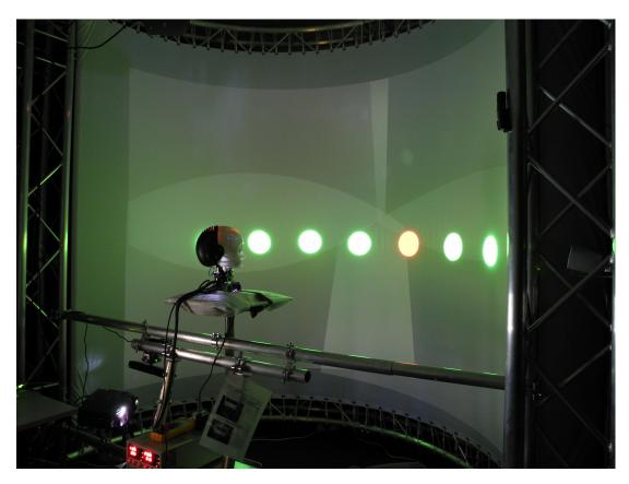
**Figure 5.3:** Setup of the loudspeakers in the audio-visual VR experimental setup. The dots represent the location of sound sources behind the screen.
