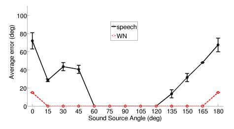
Figure 3.9: IC average errors when training with speech and testing with white noise or speech. Notice that the localisation error for white noise is zero for most angles. It is interesting to notice that training with speech produces a system that performs better than the common practice of training with white noise.
