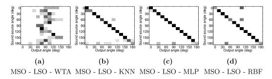
**Figure 4.7:** Confusion matrices when using MSO and LSO representations as input for WTA and the winning classification methods.
