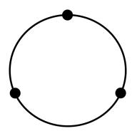
**Figure 2.1:** Array of 3 microphones in a ring. Array proposed by Huang *et al.* (1997a).
