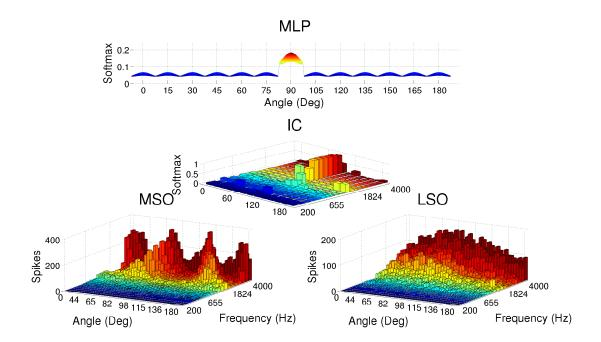
Figure 2.10: Output of all the layers in the SSL architecture for white noise presented in front of the robot  $(90^{\circ})$ . Higher frequencies are represented in red and lower in blue. Notice that for this angle most of the IC frequency components agree on the sound source angle and the MLP correctly classifies the IC output.
