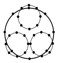
Figure 2.4: 32 microphones in a 4 rings array. Array proposed by Tamai *et al.* (2005).
