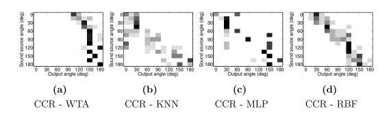
Figure 4.4: Confusion matrices when using CCR representation as input for WTA and the winning classification methods.
