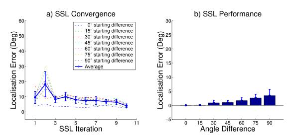
Figure 5.9: Dynamic SSL using the Soundman wooden head. a) SSL performance in consecutive iterations. The dotted curves display the performance for different angular differences at the beginning of each trial presenting a composed speech sound to the robot. The solid line shows the average of all dotted curves with the bars indicating the standard deviation. b) Accumulated angular error from all iterations in all SSL trials.
