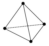
Figure 2.2: Array of 4 microphones in a pyramidal structure. Array proposed by Guentchev & Weng (1998).
