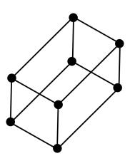
Figure 2.3: 8 microphones in a cubic array. Array proposed by Valin et al. (2003).
