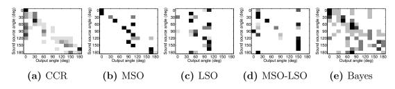
Figure A.20: SOM + RBF: Training with Speech / Testing with White Noise.
