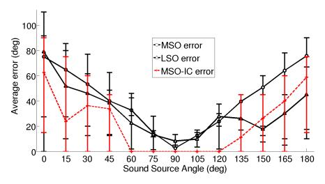
Figure 3.8: MSO, LSO and IC average errors when training with speech and testing with WN and speech. The errors are averaged over all sound classes. Notice that the IC has higher accuracy than the MSO and LSO.
