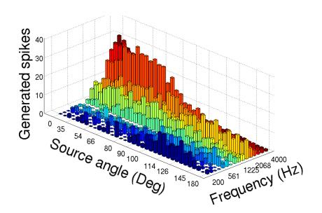
Figure 2.8: Activation of the LSO model for a sound consisting of white noise, presented to the robot at  $15^{\circ}$ . Notice that *higher frequencies* (red) are more informative, as they produce a larger concentration of neural firing in the neurones sensitive to sounds produced around  $15^{\circ}$ , which is the real sound source angle, whereas *lower frequencies* (blue) trigger the firing of neurones sensitive to sounds produced at the wrong angles.
