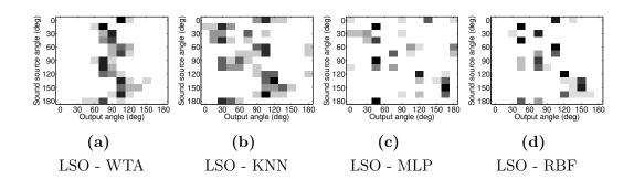
Figure 4.6: Confusion matrices when using LSO representation as input for WTA and the winning classification methods.
