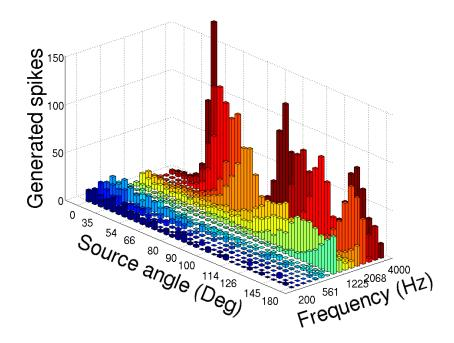
Figure 2.7: Activation of the MSO model for a sound consisting of white noise, presented to the robot at  $15^{\circ}$ . Notice that *lower frequencies* (blue) are more informative, as they produce a larger concentration of neural firing in the neurones sensitive to sounds produced around  $15^{\circ}$ , which is the real sound source angle, whereas *higher frequencies* (red) trigger the firing of neurones sensitive to sounds produced at the wrong angles.
