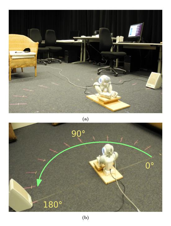
**Figure 3.1:** Sounds were played around the Nao in half circle  $\emptyset 2 \text{ m}$ , from  $0^{\circ}$  to  $180^{\circ}$  in  $15^{\circ}$  steps. 13 recordings were made in a room with reverberation damped by curtains.
