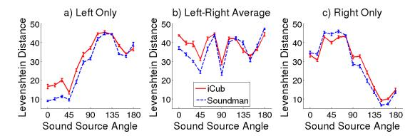
**Figure 5.7:** Average Levenshtein distances between the DASR output and the ground truth. Results obtained with both robotic heads for the frontal 180° on the azimuth plane.
