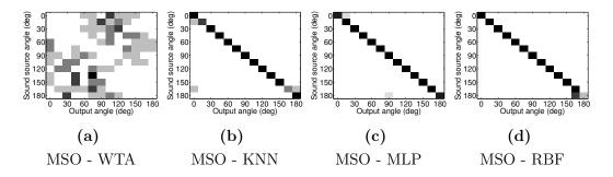
Figure 4.5: Confusion matrices when using MSO representation as input for WTA and the winning classification methods.
