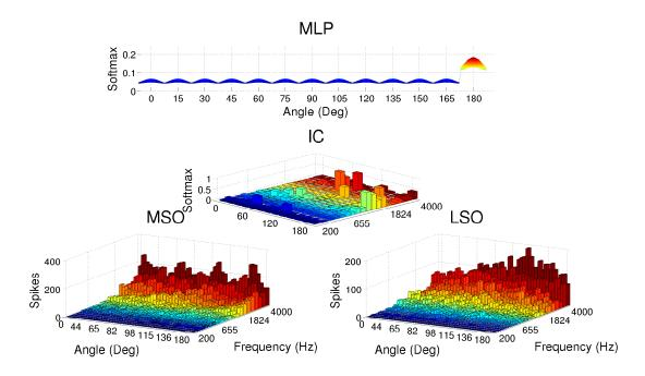
Figure 2.11: Output of all the layers in the SSL architecture for white noise presented on the right side of the robot  $(180^{\circ})$ . Higher frequencies are represented in red and lower in blue. Notice that for this angle most of the IC frequency components disagree on the sound source angle; however, the MLP can cope with these non-linearities and correctly classifies the IC output.
