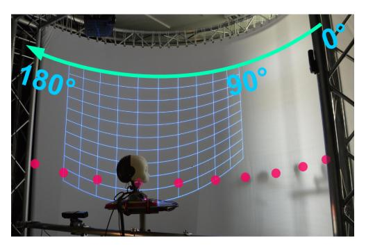
Figure 4.1: Audio-visual VR experimental setup. The grid shows the curvature of the projection screen surrounding the iCub humanoid robot head and the dots represent the location of the sound sources behind the screen.
