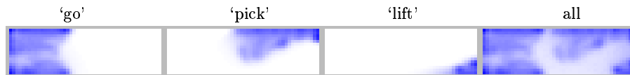
Fig. 8. Trained weights W^{td} to four selected language units of the student robot. Each rectangle denotes the hidden area, dark are strong connections from the corresponding regions. Each of the three left units is active only at one input which is denoted above. The rightmost unit is active at all language words.
