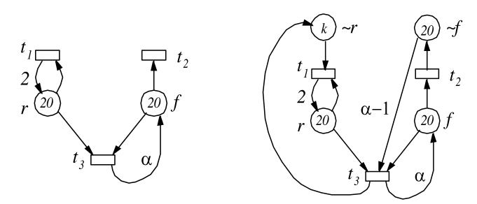
P/T models of the predator/prey system, with  $\alpha_r=0$ ,  $\alpha_f=\alpha$ ,  $\beta_r=2$ ,  $\beta_f=0$ ,  $|\Pi|=|\Delta|=20$ . They can be seen either as discrete or as continuous PN.
