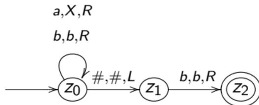
$z_0 a a b \vdash X z_0 a b \vdash X X z_0 b \vdash X X b z_0 \# \vdash X X z_1 b \vdash X X b z_2 \#$
