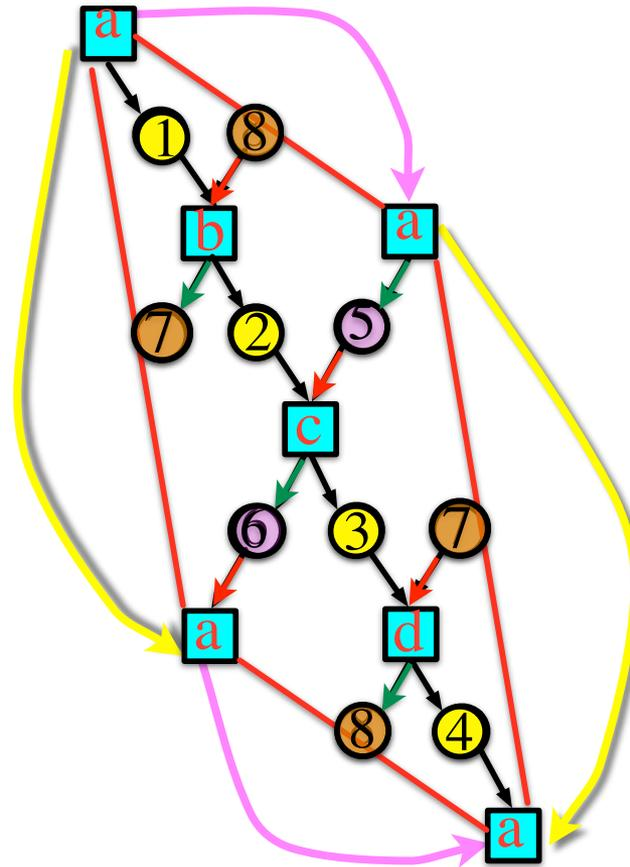
Folding the Space-Time image of a parallelogram to a „Cycloid“ represents signal movement periodic in space and time.
